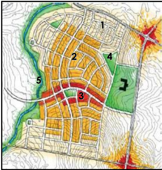
Figure 5-5: TND form: (1) Lower-density residential, (2) urban residential, (3) Mixed-Use center, (4) Open Space and Civic Site, and (5) Linear Park.
